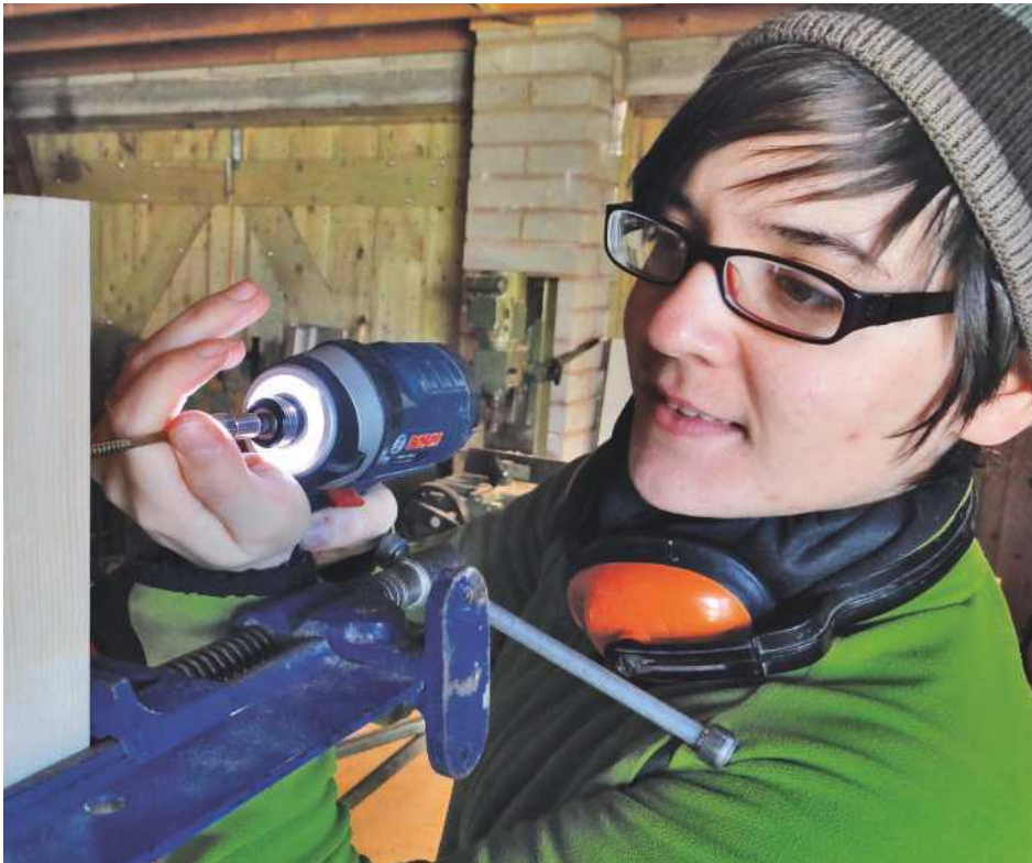
▲ Pic.1 Aurelia screwing through the leg into the end-grain of the tenon
